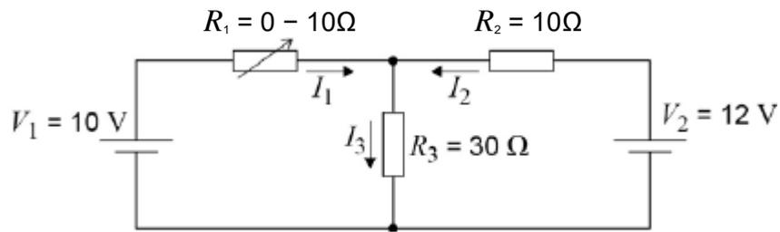
$R_1$  is a variable resistor with a resistance that varies between 0 and  $10\ \Omega$ .
