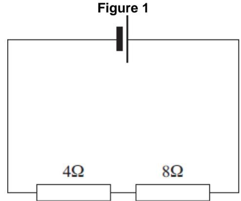
Calculate the potential difference across the 8 Ω resistor.
